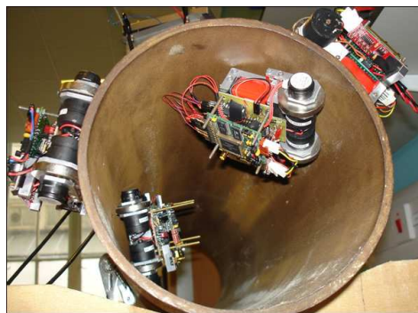
Fig. 3.3 : X-ray robots inside and outside of a pipe searching for cracks. (Source: Internet site University of Strathclyde (2006))
