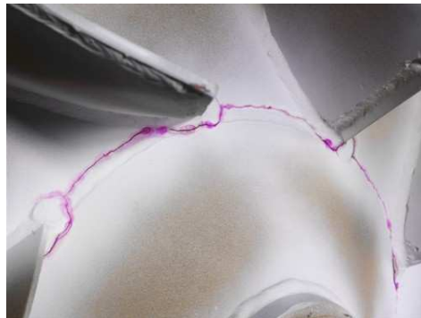
Fig. 3.1 : Dye penetration in the stiffening cone of a turbine. (Source: Internet site www.venti-oelde.de (2009))
