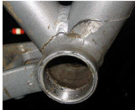
Fig. 1.7 : Crack in a bicycle crank. (Source: internet)
